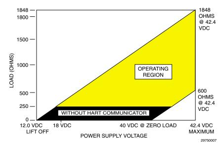
Figure 1-4. Power Supply and Load Requirements
